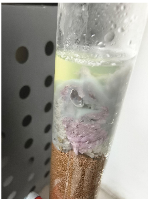
Photo 5. Supplier-provided laboratory column/test image showing retained/formed solids. Composition and uranium content require analytical confirmation [13].
