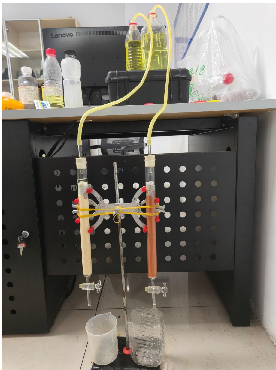
Photo 7. Supplier-provided parallel laboratory column test. The setup is useful as a qualitative process-development reference; test conditions and mass balance were not supplied [13].
